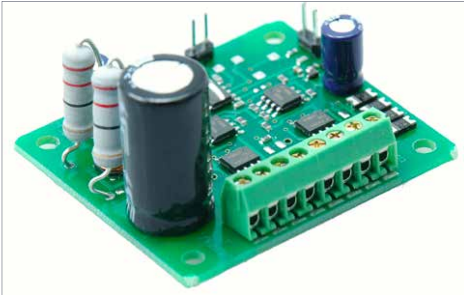
8. Digitrax has the DS52 for any style snap motor or two stall motors. Notice the large storage capacitor in the front. Digitrax photo
