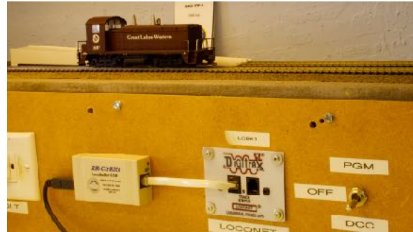
1: The programming track station and selector switch at the PebbleCreek Model Railroad Club
