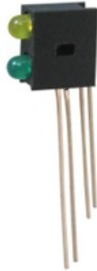
3: A bi-level LED assembly suitable for a track-side signal as is — photo courtesy of All Electronics
