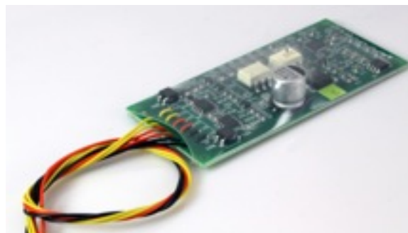
10: PTB-100 Programming Track Booster from SoundTraxx
