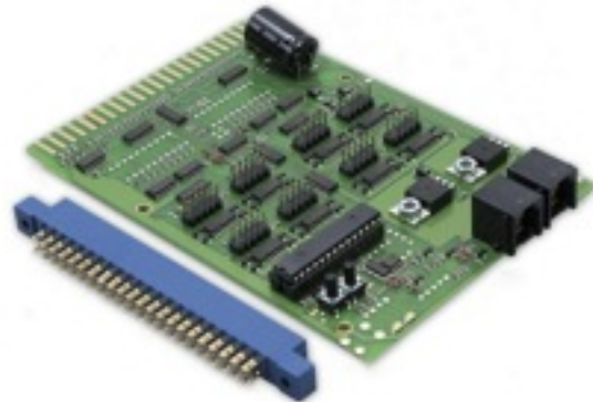
8: Digitrax SD8C Signal Decoder board — photo courtesy of Digitrax
