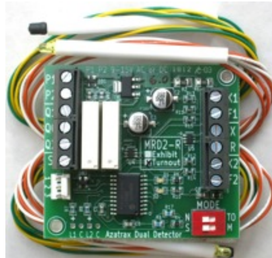
7: Azatrax MRD2 optical detector — senses two places in the block — photo courtesy of Azatrax
