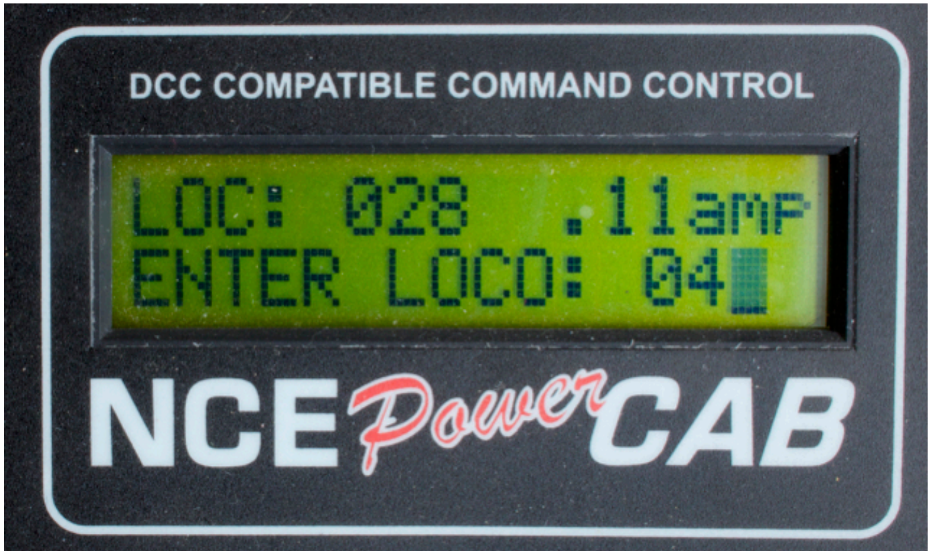
5: Inputting a long address for loco #4 (figure 1) on a NCE PowerCab by using a leading zero
