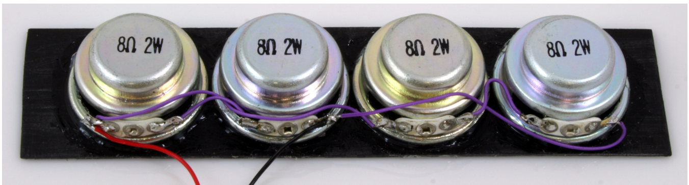
4: Line array of four identical speakers - wired in a series-parallel combination, the resulting unit is rated at 8 ohms and 8 watts.
