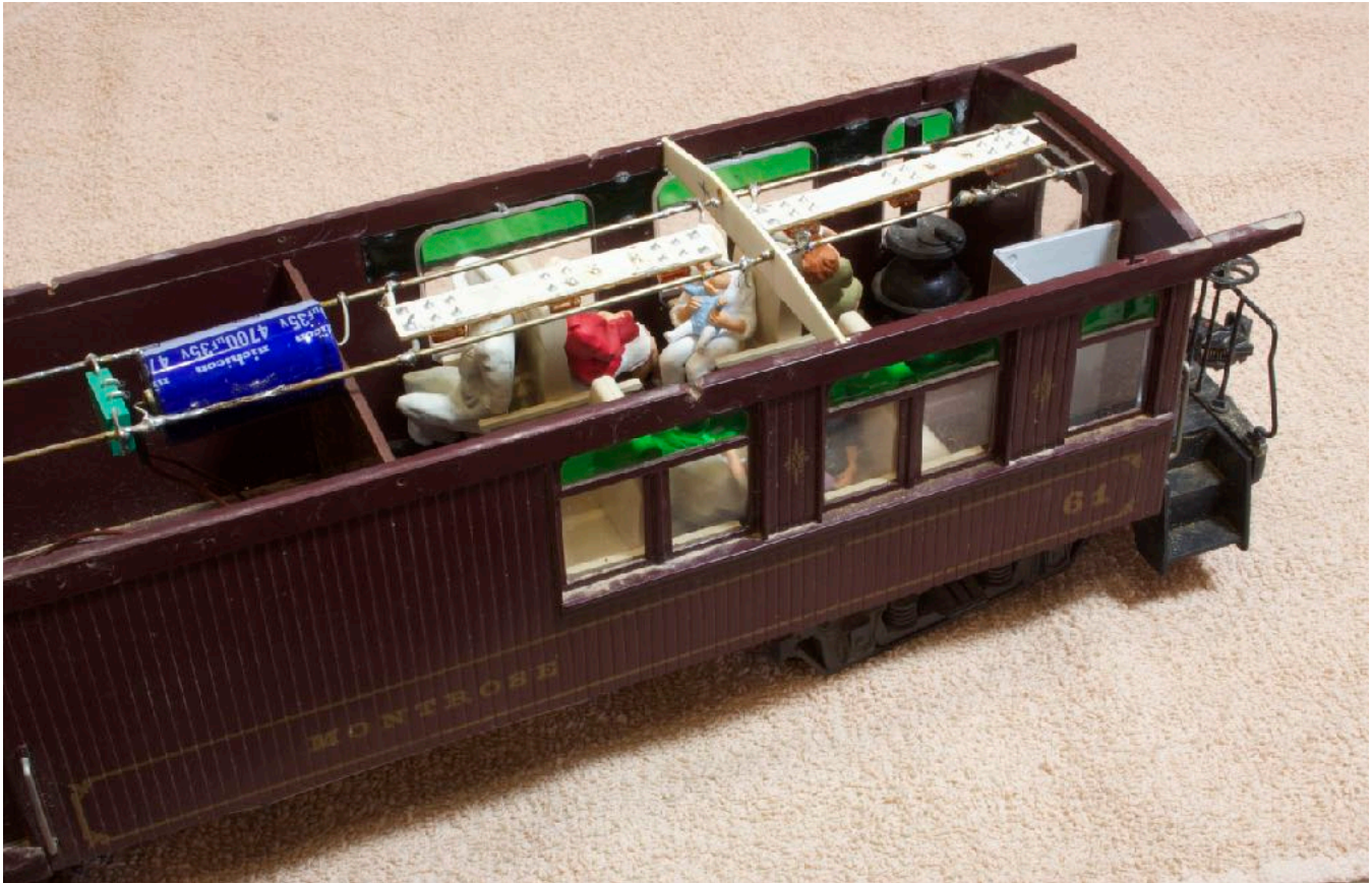
8: Lighted passenger car from figure 1 with the roof off, showing LED packages installed
