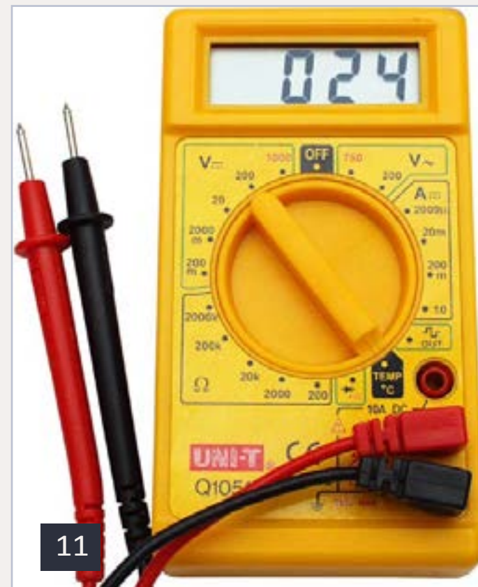
11: Digital Multimeter – photo courtesy of Litchfield Station.
