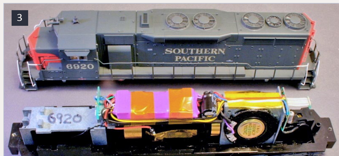
3: SoundTraxx Tsunami aftermarket installation in an Atlas SD-35 designed for sound.
