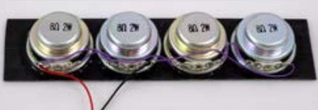
12: A series-parallel wiring of four speakers.
