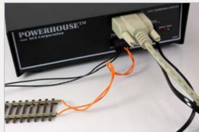
Figure 5: NCE command station with RS232 cable interface.
